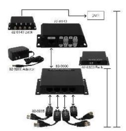
Transmit power and video signals over standard UTP CAT5 cables. The video/power balun carries DC power along with video over standard UTP cable. The built-in DC plug on the video/power balun at the camera end (#82-9300) receives power from the transmitter (#82-9295). The male BNC to RJ-45 jack converts 75ohm video to 100ohm video for use with enconomical UTP CAT5 cables.
