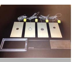
The Qi Foreign Objects are WPC defined metal objects that can be placed between Qi wireless transmitters and receivers and used to evaluate the FOD operation and performance.
