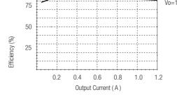
Efficiency Vs Load (Vin=Min)
