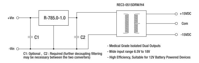
Isolated (up to 6KV), wide Input range regulated output
