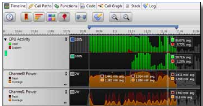
Power, current and voltage data can be displayed alongside thread activity and other performance metrics to enable energy optimization
