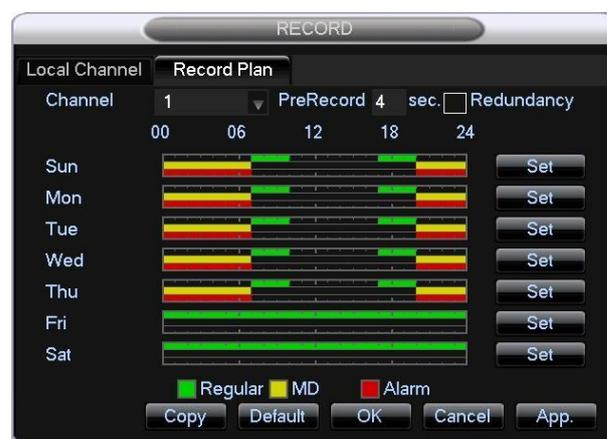
Define up to 6 time periods by entering the start and finish times for each one, and select the type of recording applicable for this period (see chapters 3.2.3 and 3.2.4 for details on these recording types).
