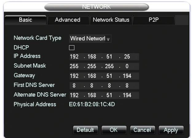
**NOTE** Please ensure **DHCP** is left unticked. If it is selected, the IP address will be automatically assigned as required, and remote connection will be delayed as the server will need to “find” the DVR again.
