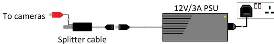
The cameras are powered via the 18m CCTV cable supplied. The cable carries both the power to the camera, and the video feed from the camera to the DVR. This setup allows you to power up to 8 cameras from a single power socket.
