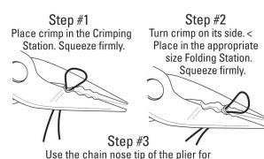
Use the chain nose tip of the plier for any additional squeezing or bending.
