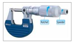
Rotating the thimble/speeder when the workpiece is between the anvil and spindle causes the ratchet mechanism to operate and apply a constant measuring force to the workpiece.
