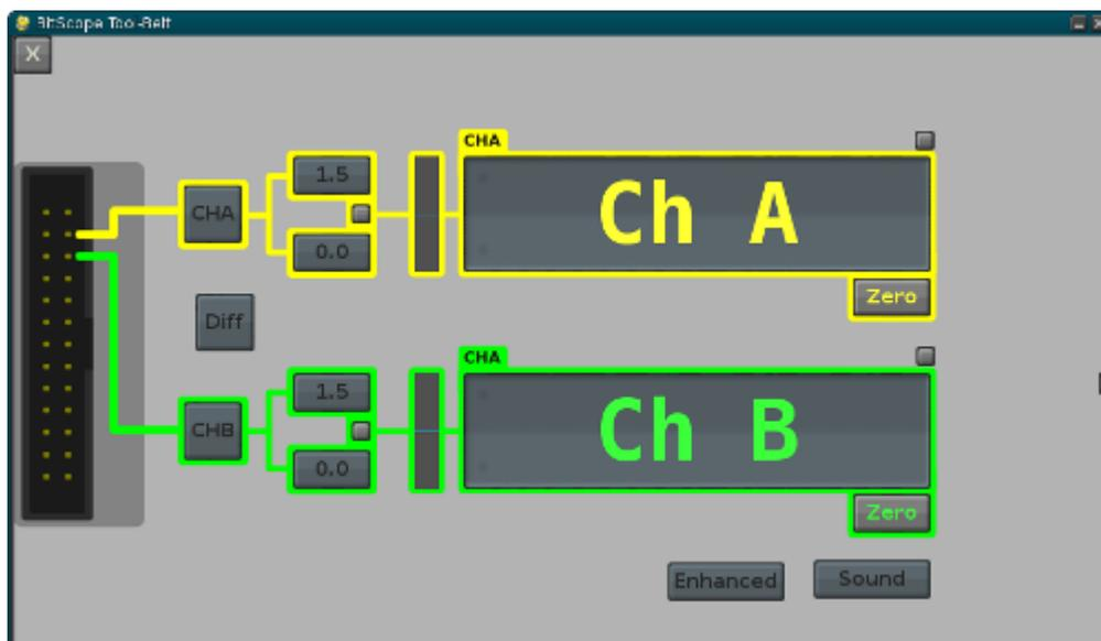
A key design goal is to simplify UI design and promote the use of many “single purpose” apps rather than fewer complex ones. Each app is designed to “do one thing well” whether it’s a multimeter, oscilloscope, waveform generator, logic or spectrum analyzer or anything else. Further, the MVC model need to not be driven by a UI; it can use a machine interface for automated testing, data acquisition, system diagnostics and process monitoring.
