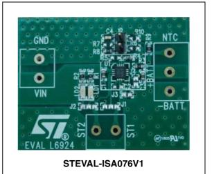
When a current-limited adapter is used, the device can operate in quasi-pulse mode, dramatically reducing power dissipation.
