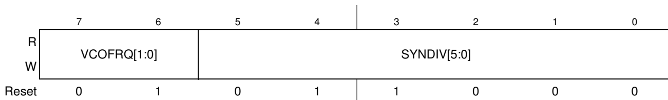
Figure 8-5. S12CPMU_UHV_V6 Synthesizer Register (CPMUSYNR)
