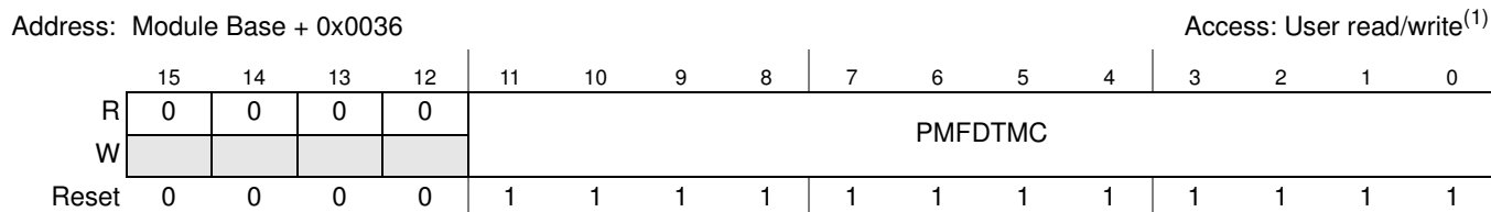
Figure 14-38. PMF Deadtime C Register (PMFDTMC)
