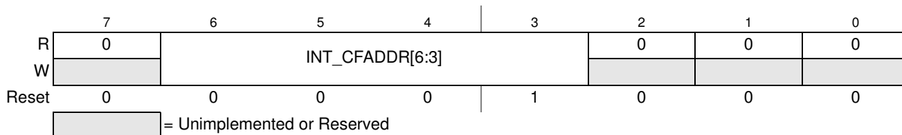
Figure 4-4. Interrupt Configuration Address Register (INT_CFADDR)
