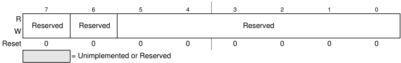
Figure 9-21. ADC Command Register 3 (ADCCMD_3)
