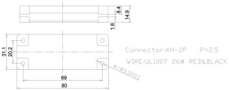
Dimensions : Millimetres Tolerance: ±0.5mm
