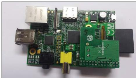
Fig. 1: R-Pi with piggy back RF-transmitter board
