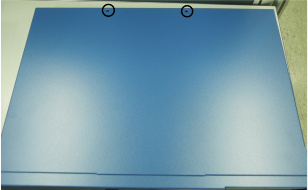
Figure 3. Removing screws from top side of chassis
