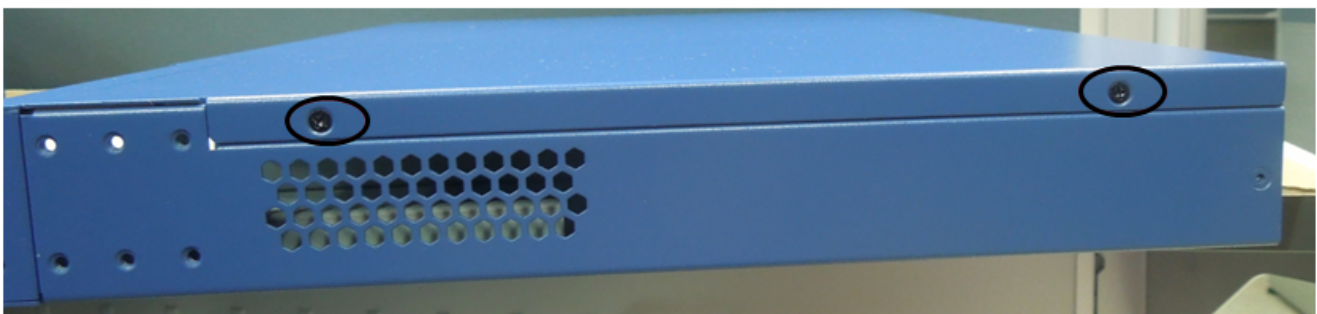
Figure 4. Removing screws from back side of chassis
