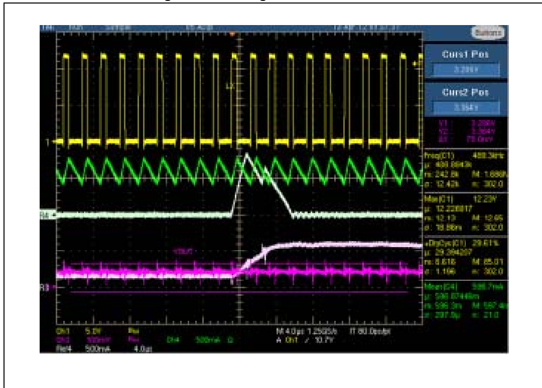
Figure 14. The regulator works in CCM
