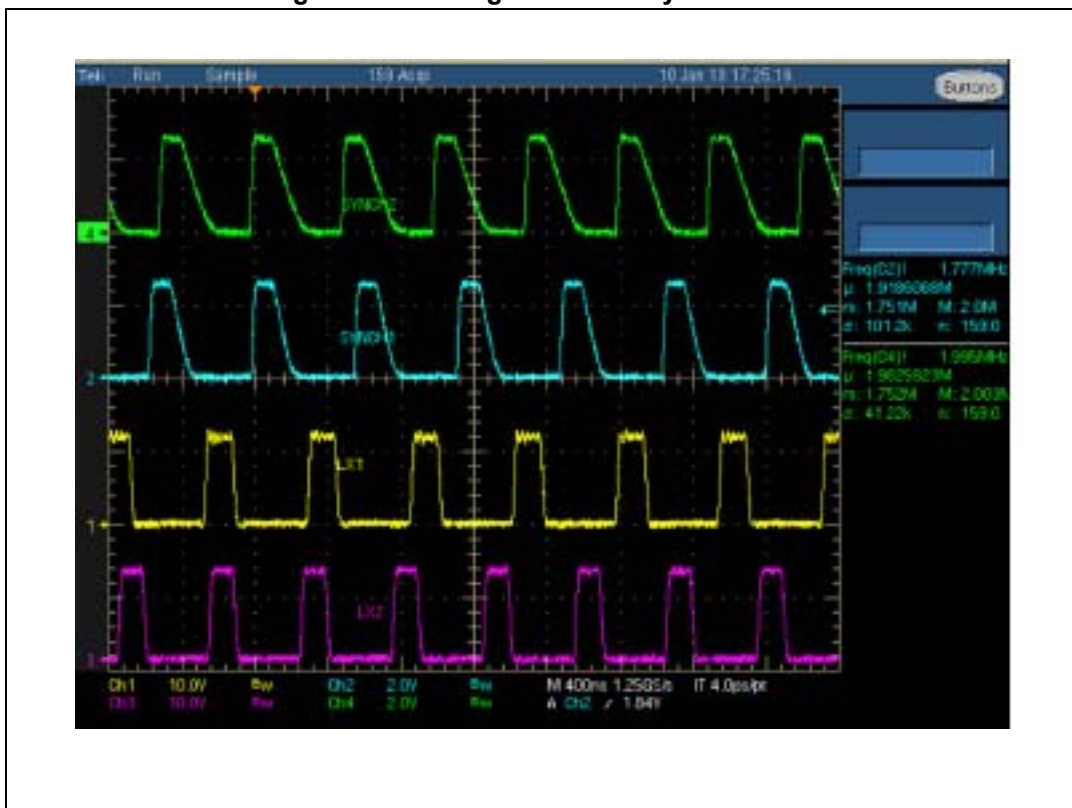
Figure 28. Two regulators not synchronized
