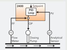
2400 series Feedforward control is excellent for chemical dosing applications
