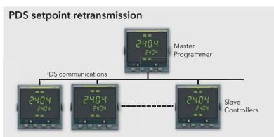
In 2000 Series controllers it is possible to use the PDS communication link to send a setpoint from one controller to a network of slave devices - providing the economical creation of multi-zone temperature control solutions.
