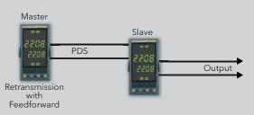
Using Eurotherm setpoint retransmission over PDS communications it is possible to use two 2400 controllers as a cascade control system with the output of the first (or master controller) forming the setpoint of the second (or slave controller).
