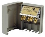
Vision New Gold masthead amplifiers are industry leading designs for amplifying very weak digital TV signals. Models V20-4260L has additional filtering to minimise the effects of 4g-LTE interference where this would cause overload in traditional masthead amplifiers. The V20-4260L employs a "mid-stage" 12dB level control which minimises noise to the weak incoming TV signal yet allows full level control.
