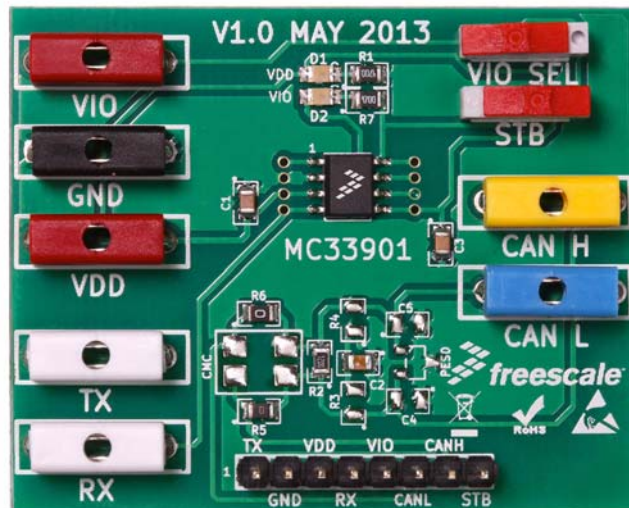
Figure 1. KIT33901EFEVB Evaluation Board
