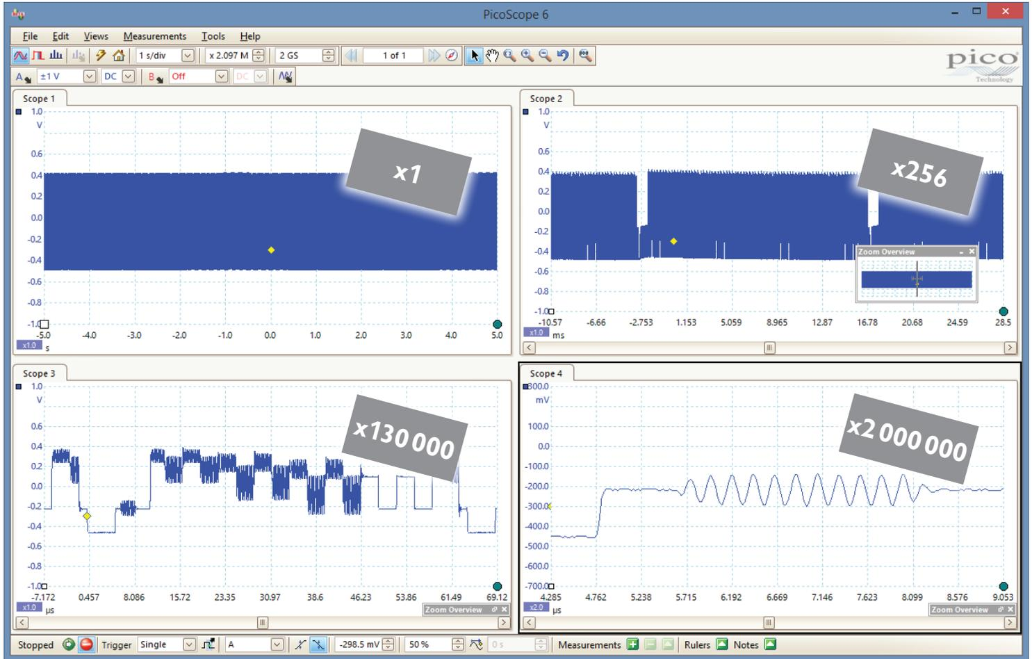
Powerful tools are included to allow you to manage and examine all of this data. As well as functions such as mask limit testing and color persistence mode, the PicoScope 6 software enables you to zoom into your waveform by several million times. A zoom overview window allows you to easily control the size and location of the zoom area.
