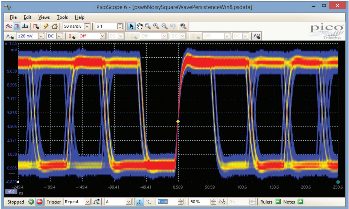
Color persistence mode allows you to see old and new data superimposed, with new data in a brighter color or shade. This makes it easy to see glitches and dropouts and to estimate their relative frequency. Choose between analog persistence and digital color, or create custom display modes.
