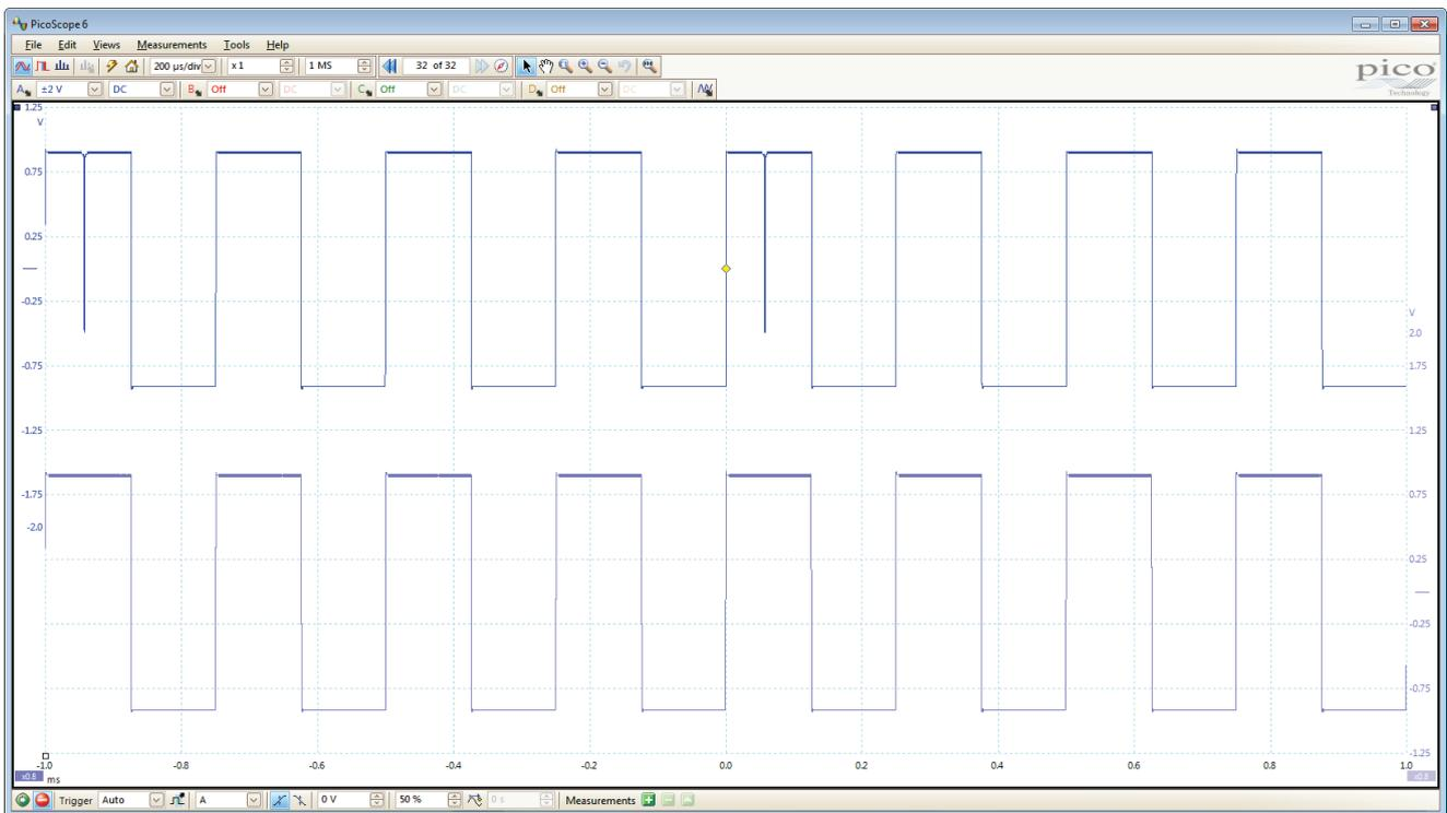
In the example above, both waveforms show the same signal, but using different types of hardware acceleration. The top waveform has used the aggregation possible with a PicoScope, and as a result the high-frequency spikes are preserved. The bottom waveform has used traditional decimation, and shows a loss of signal data.
