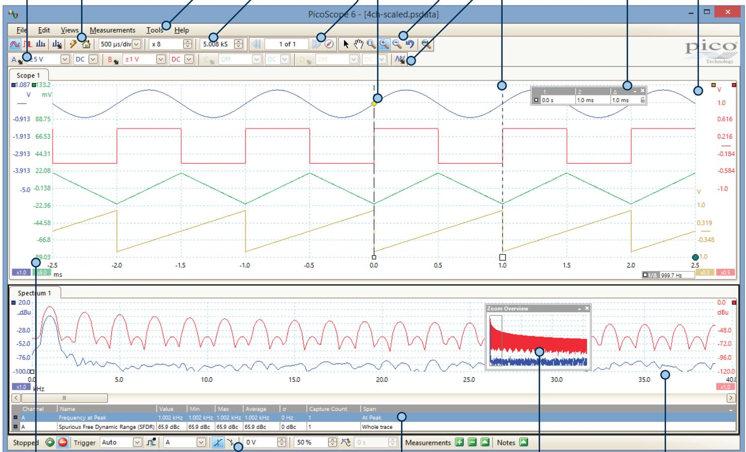
**Movable axes:** The vertical axes can be dragged up and down. This feature is particularly useful when one waveform is obscuring another. There's also an **Auto Arrange Axes** command.
