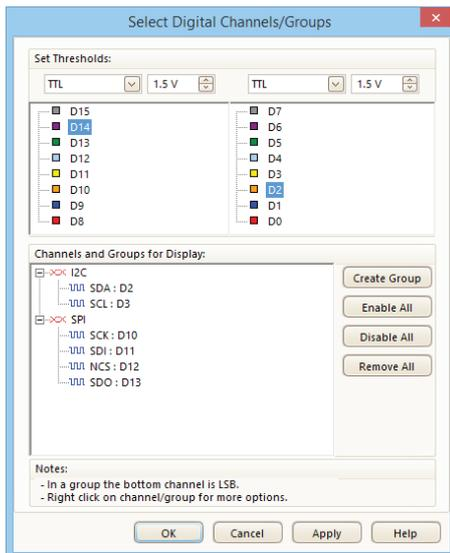
The 16 digital inputs can be displayed individually or in arbitrary groups labelled with binary, decimal or hexadecimal values. A separate logic threshold from  $-5\text{ V}$  to  $+5\text{ V}$  can be defined for each 8-bit input port. The digital trigger can be activated by any bit pattern combined with an optional transition on any input.
