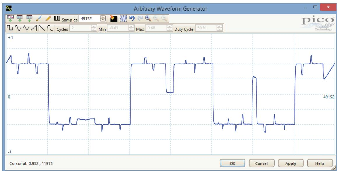
The AWG can be used to emulate missing sensor signals during product development, or to stress test a design over the full intended operating range.
