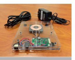
The Qi FOD Transmitter is a V1.1 power transmitter that can be used to test the operation and performance of Qi V1.1 power receiver devices. A USB serial interface is used to display operating information and to program transmitted power offsets as well as change the operating modes.
