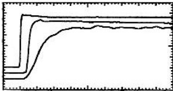
20%/div Top to bottom: 500 ps/div, 100 ps/div, and 20 ps/div 10 ps Step Response
