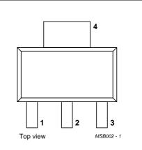
Fig.1 Simplified outline (SOT223) and pin configuration.
