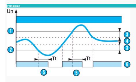
MUSF relays operate in window mode : they check that the controlled voltage stays between a minimum and maximum threshold.
