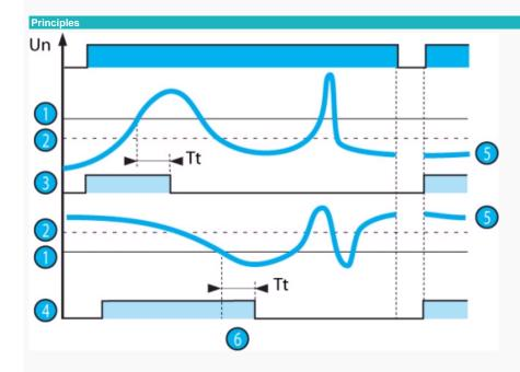
The under or overvoltage threshold value is set by a graduated potentiometer by reading the Un scale to be monitored directly.
