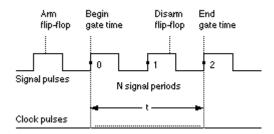
The **P6000A** measures frequency or period by counting the number of 11.059 MHz clock pulses during an actual gate time t, which corresponds to an intergral number of signal periods N. This technique allows high-accuracy low-frequency measurements. Frequency is calculated from N/t, period from t/N.
