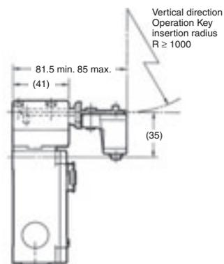
**Note: 1.** Unless otherwise specified, a tolerance of  $\pm 0.4$  mm applies to all dimensions.
