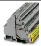
Installation ground terminal block, Cross section: 0.2 mm² - 4 mm², AWG: 24 - 12, Connection type: Screw connection, Width: 6.2 mm, Color: gray, Mounting type: NS 35/7,5, NS 35/15
