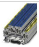
Protective conductor double-level terminal block, Cross section: 0.08 mm² - 4 mm², AWG: 28 - 12, Connection type: Spring-cage connection, Width: 5.2 mm, Color: gray, Mounting type: NS 35/7,5, NS 35/15
