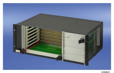
■ CompactPCI chassis with 48 V<sub>DC</sub> power supply
