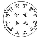
Terminal numbers molded on bottom of housing.
