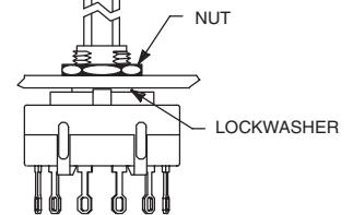
Install switch with stop ring (if used) and lockwasher in back of panel. Tighten hex nut from front of panel.
