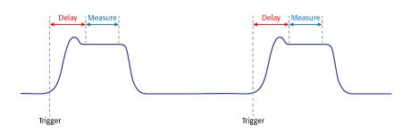
Series 2280S power supplies enable time-critical measurements on fast-changing or pulse-like loads. An external trigger initiates the acquisition. Programmable delay and measure times enable measurements at a specific time on the load current pulse such as when the peak has stabilized.
