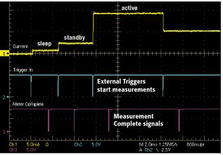
Series 2280S power supplies measure the start-up load currents as a device powers up. An external trigger tells the Series 2280S when to make a measurement. The Series 2280S signals when the measurement is completed so that the device can be put in its next state.
