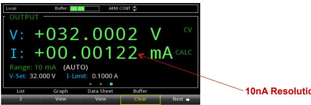
With its flexibility for controlling the number of power line cycles for the measurement and ability to use filtering, the Series 2280S can measure very low currents down to 100nA.
