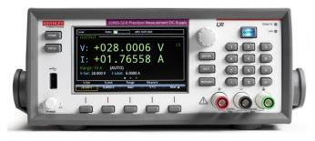
Keithley's Series 2280S Precision Measurement, Low Noise, Programmable DC Power Supplies can source stable, low noise voltages as well as monitor load currents over a wide dynamic range from amps to 100 nanoamps. The Model 2280S-32-6 can output up to 32V at up to 6A; the Model 2280S-60-3 can output up to 60V at up to 3.2A.
