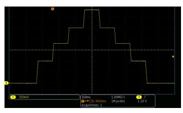
**List Mode** automatically steps the voltage through the programmed steps. With the Series 2280S supplies, the output can be displayed using the internal graphing capability.
