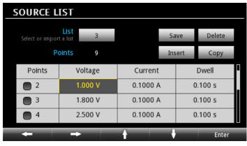
Create a test consisting of a number of output voltage levels using the Series 22280S' **List Mode** setup screen. Alternatively, download a list using a USB flash drive.
