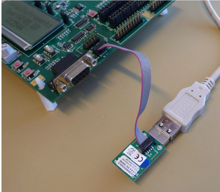
Figure 12 - CC2544 USB Dongle connected to SmartRF05EB
