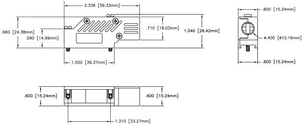
Dimensions : Inches (Millimetres) Tolerance: ±0.020 [0.508]
