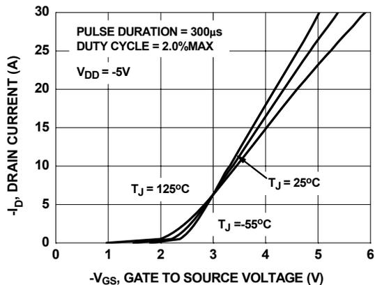
**Figure 5. Transfer Characteristics**
