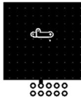
a.  $60^\circ\text{C}/\text{W}$  when mounted on a 1 in<sup>2</sup> pad of 2 oz copper
