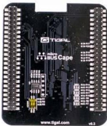
The dip-switch “ADDR” in the bottom of the Cape allow user to modify I2C address of the EEPROM, this is useful in case of conflict or cascade of Capes. The two pin represent the last two bits of the address so the allowable address range is composed of four address, from 0x54 to 0x57 (default 0x57).
