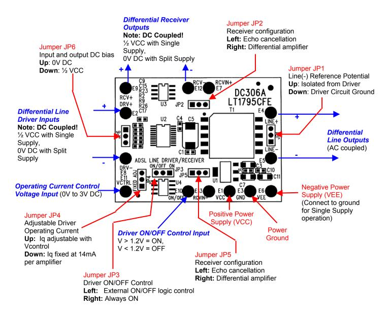
Posts E7 and E13 are test points. These points allow monitoring the signal at the the primary of the line coupling transformer.
