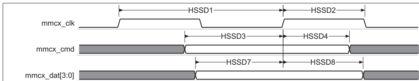
Figure 6-65. MMC/SD/SDIO – High-Speed SD Mode – Data/Command Receive
