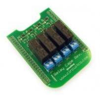
The Relay Cape provides 4 3 amp capable relays with screw terminals. The relays are SPST, Normally Open. They are driven from GPIO lines.
