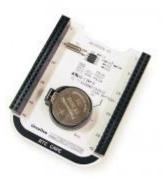
The RTC Cape provides time tracking capability for the BeagleBone Black even when the power is lost. This cape features the DS1338 I2C-based real-time clock/calendar and a holder for a coin battery type CR2032. Setup, reading, and setting up time is easy with the provided device tree overlay.
