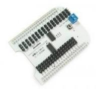
Picture Coming Soon The PWM Cape provides 32 channels of PWM output, addressed over an I2C interface. The three pin connectors are wired in a standard servo pinout, and power to the connectors can be provided from a screw terminal block on the end of the board.
