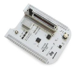
The Bacon Cape is an accessory board design to be used with the BeagleBone Black or original BeagleBone (aka White). The Bacon Cape was designed to provide hardware examples of some of the basic input/output features of the BeagleBone products.
