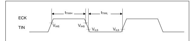
• Trigger input timing
