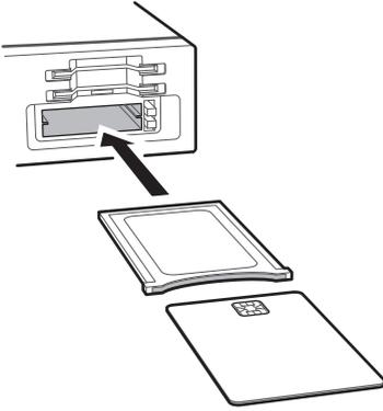
To watch Conax-scrambled pay channels, insert a Conax pay-TV card into the card slot. To watch non-Conax channels, insert a pay-TV card into a CA module, and then insert the CA module into the CAM slot.
