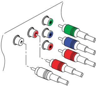
The receiver's component video connectors are labelled Y, Pb, and Pr, and their companion audio connectors are labelled L and R. Each of them is coloured differently. A typical component cable has five connectors. Connect the receiver's component video and audio output connectors to the TV's component video and audio input connectors using a component cable, so that the connectors of the same colour connect to each other.
