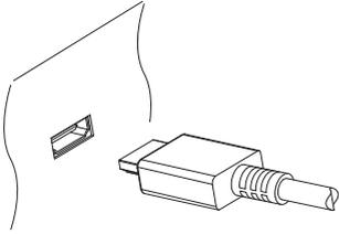
Connect the receiver's HDMI output connectors to the TV's HDMI input connector using an HDMI cable.
