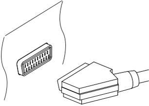
Connect the receiver's SCART output connector to the TV's SCART input connector using a SCART cable. An extra audio connection is not needed because SCART also carries audio.
