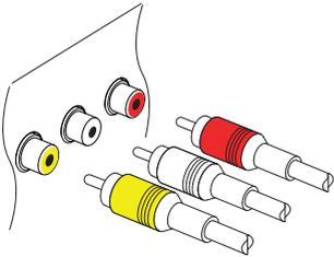
The composite video connector shares the audio connectors with the component video connectors. A typical composite cable has three connectors. The yellow connector is for the video connection. Connect the receiver's composite video and audio output connectors to the TV's composite video and audio input connectors using a composite cable, so that the connectors of the same colour connect to each other.
