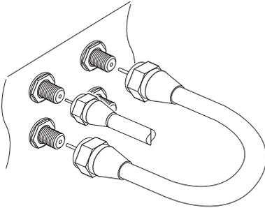
Connect the cable from the satellite dish to LNB IN 1. In most situations, connect LNB OUT 1 to LNB IN 2 using the loop-through cable. Only when two satellite dishes are available without any multi-dish switch, users should connect the cable from the other dish to LNB IN 2
