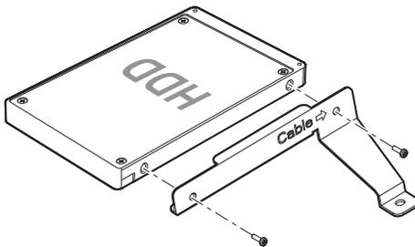
4. Place the hard drive on the receiver base, aligning the holes for the screws, and fasten the screws.
