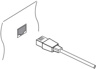
Connect the receiver's LAN port to the router using a network cable. For details on how to configure the network settings, see [Network Settings](#) on page 57.
