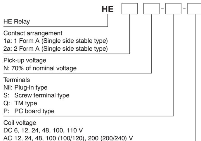
**TYPES****1. PC board type (1 Form A, DC coil) (Single side stable)**
