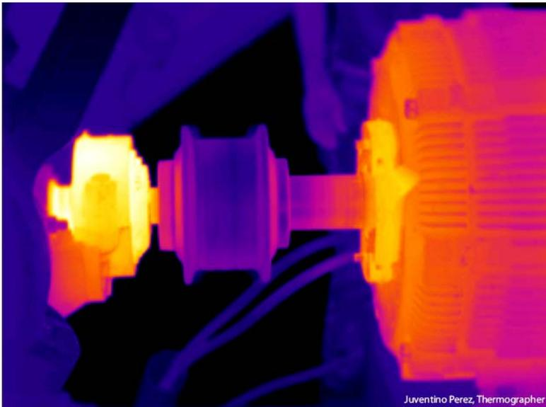
1. When machines are misaligned the flexible couplings begin to heat up and the machine operates at higher temperature, especially around the bearings.
