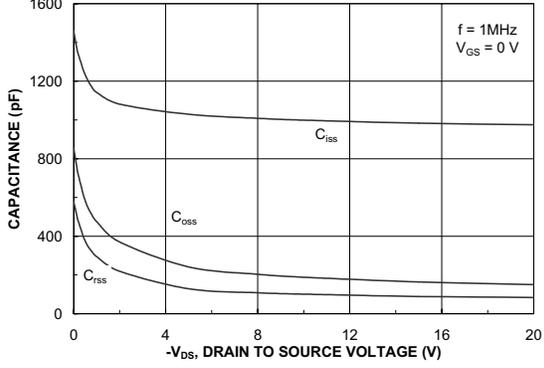
**Figure 8. Capacitance Characteristics.**
