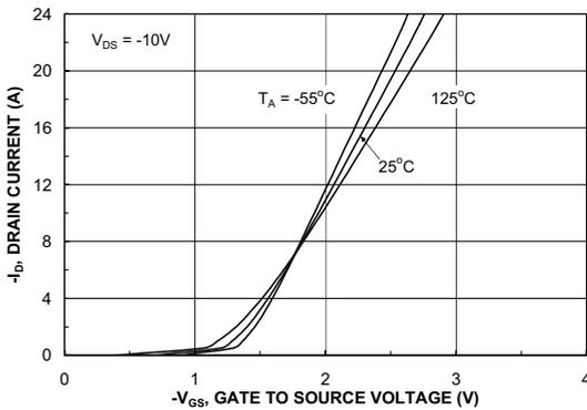
Figure 5. Transfer Characteristics.
