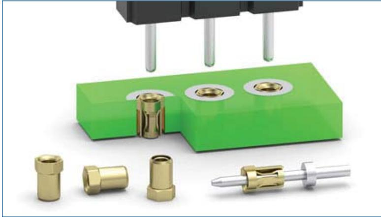
Mill-Max is pleased to announce a new option in our receptacle line-up with the introduction of a new receptacle providing flush mount PCB assembly and dual entry capability.
