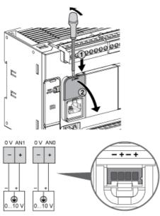
The (-) poles are connected internally.
