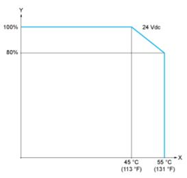
X: Ambient temperatureY: Input simultaneous ON ratio
