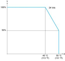
X: Ambient temperatureY: Input simultaneous ON ratio
