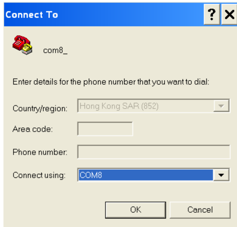
Figure 16. Connect using USB-RS232 Com Port
