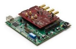
Texas Instruments in collaboration with Xilinx developed a triple-rate SDI and video clocking daughter card for the Xilinx Spartan-3A/3E development kits. The daughter card plugs directly into the Spartan development board through an EXP connector. The combined solution of the daughter card and the development kit provides broadcast video system designers a comprehensive platform for rapid evaluation and prototyping of new designs to reduce time to market.
