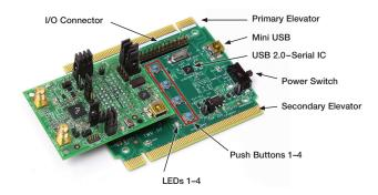
Connect the TWR-RF-MRB USB connector (J2) to the USB of the PC.
