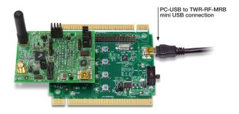
To run the board mounted on TWR-RF-MRB, configure J17 with jumpers: 2–3, 5–6, 7–8–9 (any position), 11–12, 14–15.
